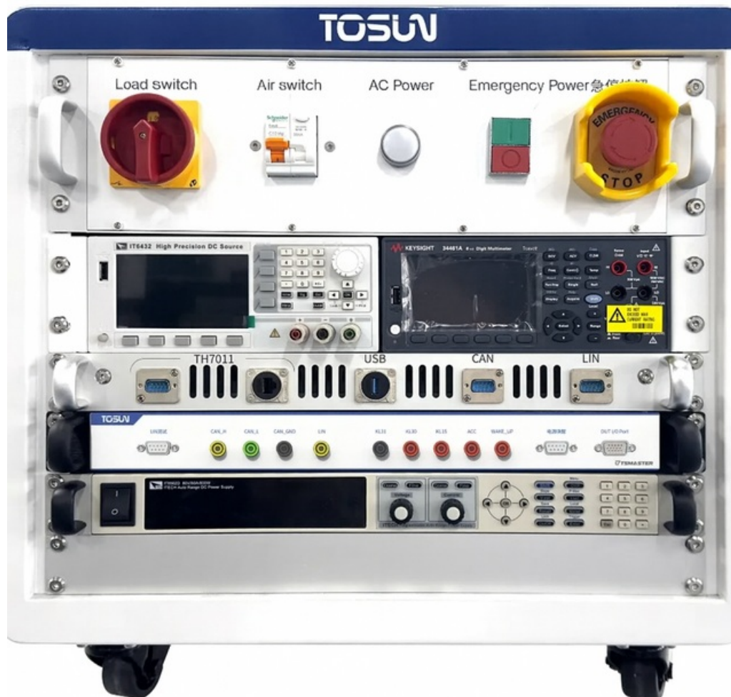
Figure 1: The TOSUN CAN FD/CAN Bus Conformance Test System rack cabinet.
