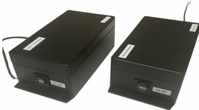
Figure 1: Field programmer USB 3.1 connector on the rugged enclosure.
