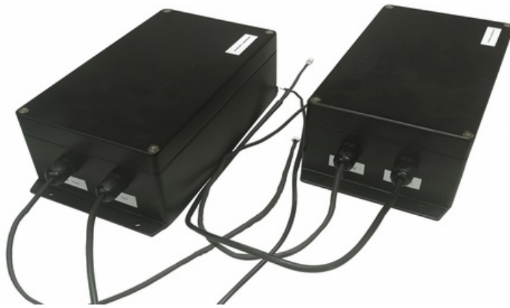
Figure 2: Field programmer JTAG and auxiliary cables connected to the rugged enclosure.
